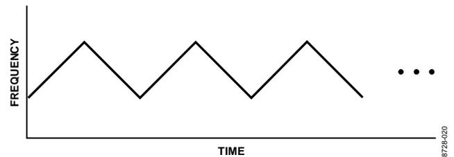
Figure 30. Continuous Triangular Ramp
