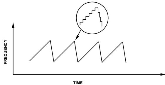
Figure 40 Fast Ramp Mode
