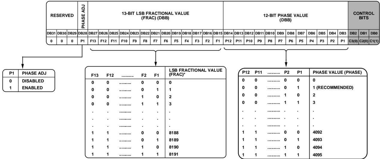
\*THE FRAC VALUE IS MADE UP OF THE 12-BIT MSB STORED IN REGISTER 0, AND THE 13-BIT LSB REGISTER STORED IN REGISTER 1. FRAC VALUE = 13-BIT LSB + 12-BIT MSB x 2<sup>13</sup>.
