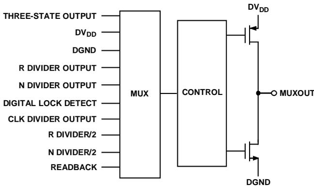
Figure 15. MUXOUT Schematic
