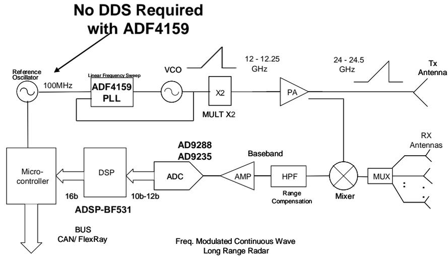
Figure 47. FMCW Radar with ADF4159
