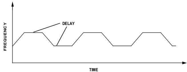
Figure 37 Delay between ramps for clipped triangular mode
