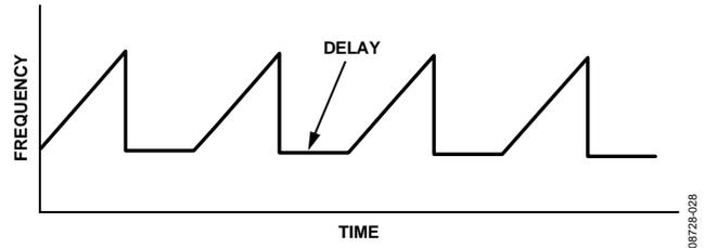
Figure 35. Delay Between Ramps for Sawtooth Mode
