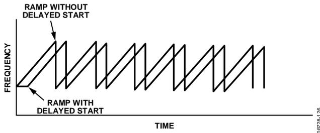
Figure 34. Delayed Start of Sawtooth Ramp
