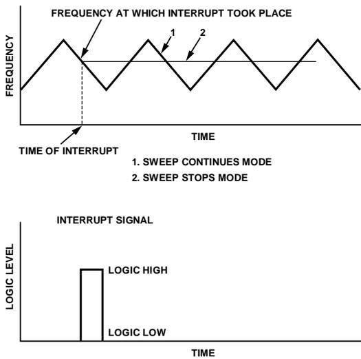
Figure 42. Interrupt and Frequency Readback
