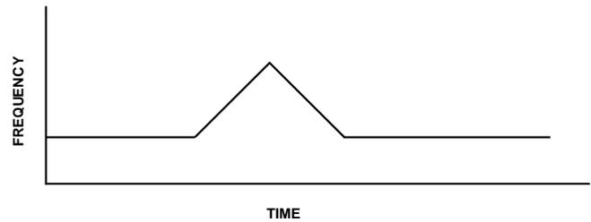
Figure 27 Single Triangle Burst
