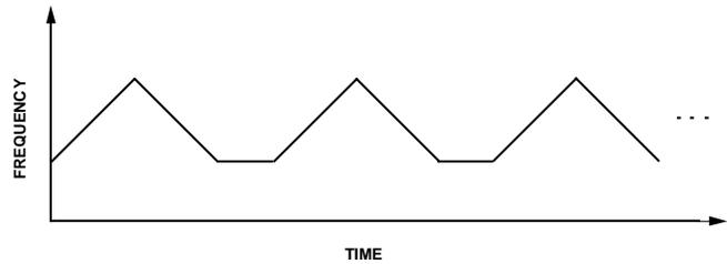
Figure 36 Delay between ramps for triangular mode
