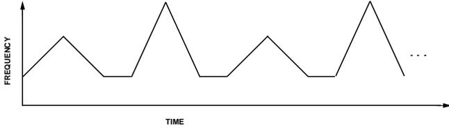
Figure 38 Two Ramp Rates Mode with Delay
