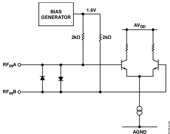
Figure 12. RF Input Stage
