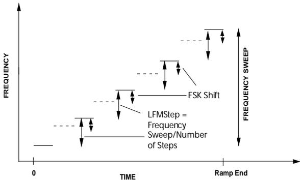
Figure 33. Combined FSK and LFM Waveform (N Corresponds to the Number of LFM Steps)
