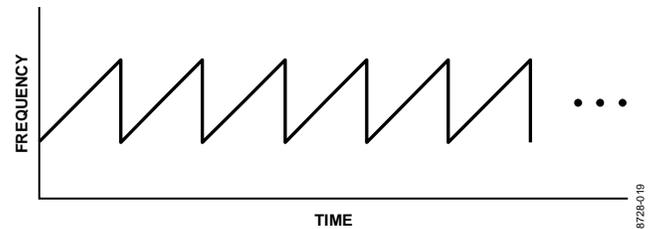
Figure 29. Continuous Sawtooth Ramp
